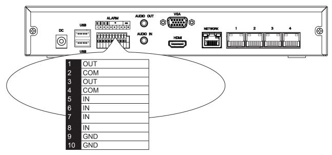
The GND are common ground for the DIs.
