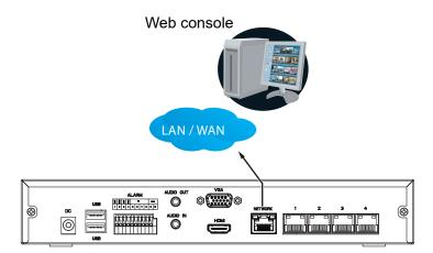
Note that when accessed over the network, the total streaming throughput is 24Mbps.
