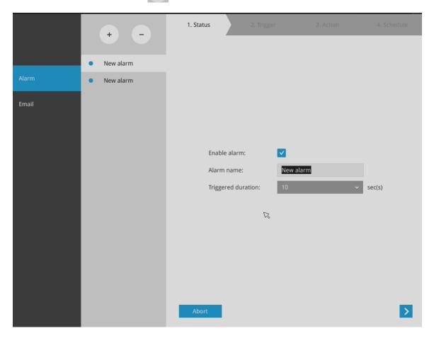
You can manually enter a name for the current setting. You can enter up to 16 numeric or alphabetic characters for the name, including symbols such as [0-9][a-z][A-Z][\_][]. You can also designate the interval between one alarm and the next triggered alarm to avoid the situation that the alarms can be too frequently triggered.
