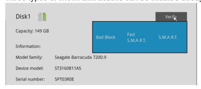
Note that disk verify function requires a volume to be temporarily disabled; namely, the video recording will be stopped before disk verify can be performed.
