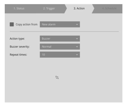
If events of different importance are issued at the same time, e.g., one major and one minor event, system will ignore the minor event and sound the buzzer tone for the major event only. The buzzer can be sounded either by the Alarm actions or the system events. If Alarm actions and system service events occur at the time, Alarm actions have the higher priority.
