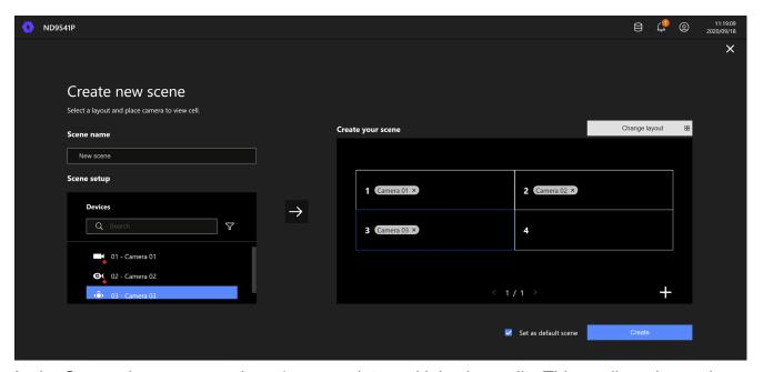
In the Scene view, you can place 1 camera into multiple view cells. This applies when using cameras with a wide coverage area, such as fisheye or multi-lens cameras.
