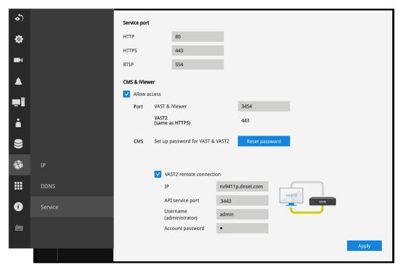
Instead of a web console, you can also access the NVR and the subordinate cameras using the **iViewer** and VIVOTEK's **VAST** software. The NVR can be managed as one of the sub-stations in a hierarchical device structure.
