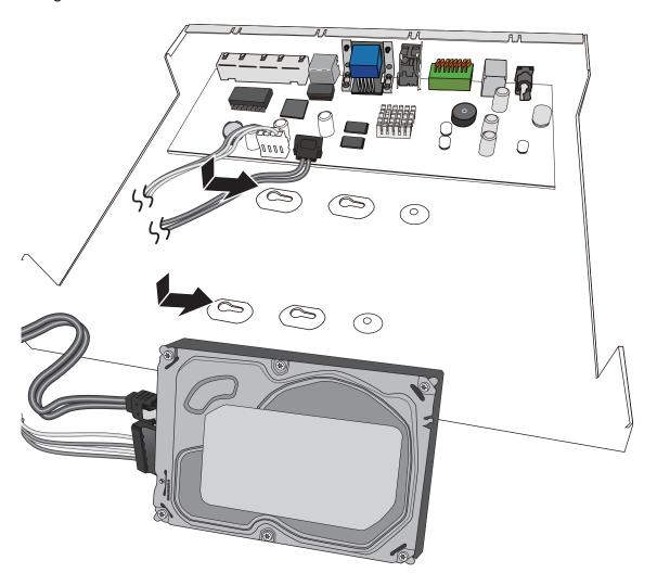
When securing screws to the hard drives, do not completely fasten the screws. Fasten the screws half way and insert the screw heads into the key slot holes. When they are in place, fasten the screws from the bottom of the chassis.
