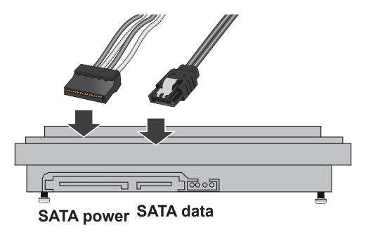
6. Install the hard drive to the chassis. Note that the screws pass through the bottom of the chassis and secure the hard drive using the mounting holes at the bottom of hard drives. When installing hard drives, their label side should be facing up, and the connector side facing the outside of the chassis.
