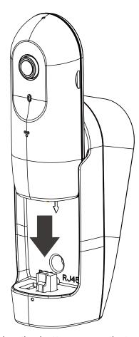
5. Use the bottom cover that comes with adhesive to seal the bottom of your device.
