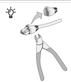
It is recommended to use an Ethernet cable without the connector jacket.
