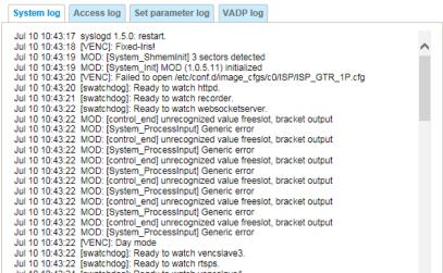
This column displays the system log in a chronological order. The system log is stored in the Network Camera's buffer area and will be overwritten when reaching a certain limit.
