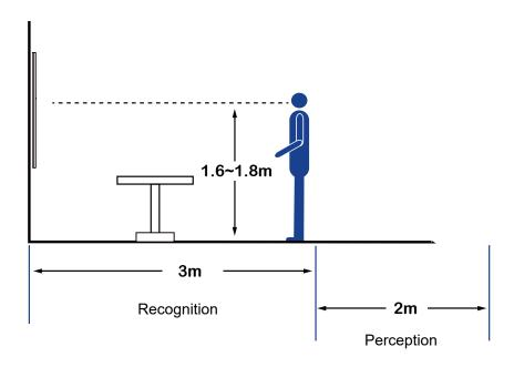
The camera is designed to capture human activities in a near-heminspheric field of view, at a place such as the entrance to a business facility. Due to the optical characteristics of wide-angle lens, image quality decreases as distance from an object increases. It is therefore recommended to install the camera within 3 meters or closer to the objects of your interest. The focus center should also be aligned with objects of importance, say, human faces.
