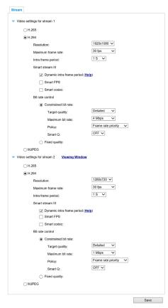
This Network Camera provides real-time H.265, H.264 and MJPEG compression standards (Triple Codec) for real-time viewing. If the H.265 or H.264 mode is selected, the video is streamed via RTSP protocol. There are several parameters through which you can adjust the video performance:
