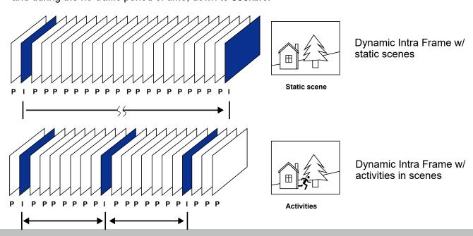
With the H.265 codec in an optimal scenario and when Dynamic Intra frame is combined with the Smart Stream function, an 80% of bandwidth saving can be achieved compared with using H.264 without enabling these bandwidth-saving features.
