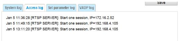
Access log displays the access time and IP address of all viewers (including operators and administrators) in a chronological order. The access log is stored in the Network Camera's buffer area and will be overwritten when reaching a certain limit.
