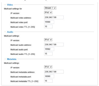
Unicast video transmission delivers a stream through point-to-point transmission; multicast, on the other hand, sends a stream to the multicast group address and allows multiple clients to acquire the stream at the same time by requesting a copy from the multicast group address. Therefore, enabling multicast can effectively save Internet bandwith.
