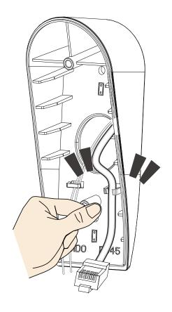
4. Slide the camera from top to bottom agrainst the bracket. The RJ45 connector should be connected.
