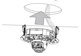
8. Use a #2 Phillips screwdriver to move the clamping plates down so that the ceiling/board is caught between the clamps and the flange on the other side of the ceiling.
