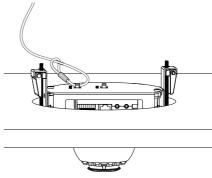
You may also use a cable tie to secure cables to the anchor point on top.
