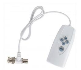
The UTC (Up the Coax) Controller is used with the GENESIS-3s series of cameras to switch between HDCVI, HDTVI, AHD & CVBS video formats to suit the requirement of the recorder on site. This is beneficial when the current video format of the camera is not compatible with the recorder.
