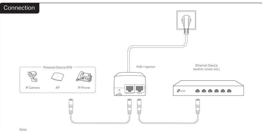
1. The PoE Injector supplies steady power and data connectivity to a powered device such as PoE IP Camera, PoE AP and PoE IP Phone through an Ethernet cable.
