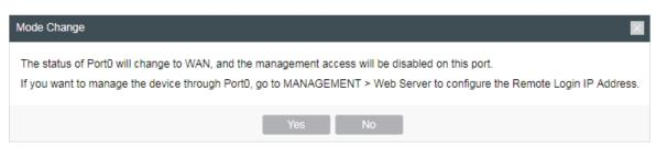
Note that if you select AP Router as the operation mode, the status of PortO will change to WAN, and the management access will be disabled on this port after the process of quick setup. If you want to manage the device through PortO, configure the Remote Login IP Address. For details, refer to 6.5. *Configure Web Server*.
