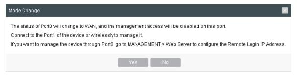
Note that if you select AP Router as the operation mode, the status of PortO will change to WAN, and the management access will be disabled on this port after the process of quick setup. You can connect to the Port1 of the device or wirelessly to manage it. If your want to manage the device through Port0, configure the Remote Login IP Address. For details, refer to 6.5. Configure Web Server.
