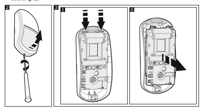
3. Install the battery and add the detector to the wireless system (see the ABAX 2 / ABAX controller manual or the INTEGRA 128-WRL control panel installer manual). The sticker with serial number which shall be entered when registering the detector in the system can be found on the electronics module.
