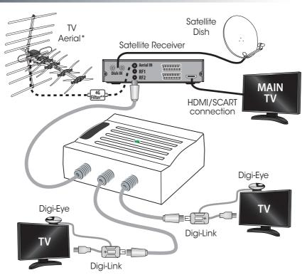
\*To distribute terrestrial TV channels over RF2 you will require a TV aerial connected to the "Aerial In" socket on the satellite receiver
