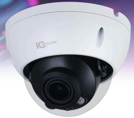
The OPTIC-6s-DM5-IV-W is 5MP motorized IP67/IK10 Vandal Proof Lite AI Dome with basic starlight technology. It has a Smart IR Viewing Distance of up to 30m and 120dB rated True WDR. Basic starlight technology offers low-light performance for applications with a minimum illumination of 0.008 to 0.009 lux, ideal for moderately dark areas such as those with streetlight coverage. With True 120db WDR on the camera, it helps provide even illumination to all areas within a scene.
