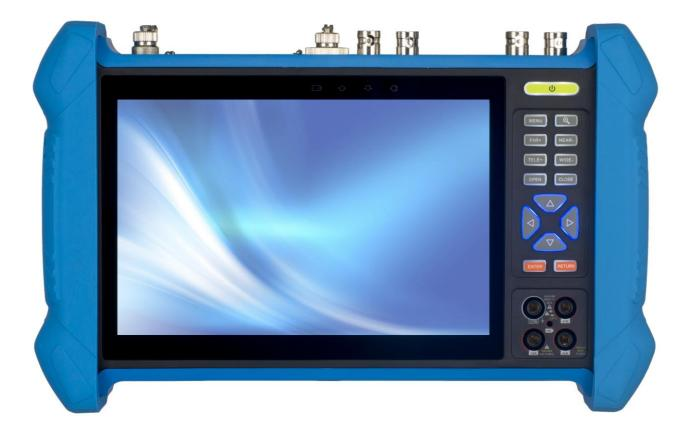
A series of T1 products uses a highly flexible rubber protective cover on both sides to protect the equipment. It not only makes your hand comfortable, but also prevents the accidental fall from damaging the equipment and reduces the impact frequency of the interface. Besides, we added a key backlight on the right side, which can help users accurately find the key in the dark environment.
