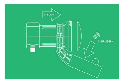
**3.** Roughly align the polarisation angle of the LNB (Astra 28.2) then connect your meter for the final fine tuning. When aligned tighten the screw on the collar.
