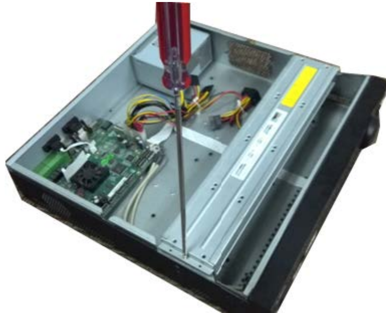
Figure 3-37 Open the top cover
