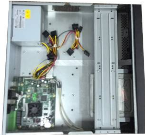
Figure 3-45 Put bracket back
