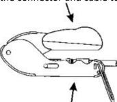
4. Release the handles and remove the connector. The cable and connector and should now be joined.
