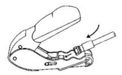
3. Squeeze the handles to compress the connector and cable together.
