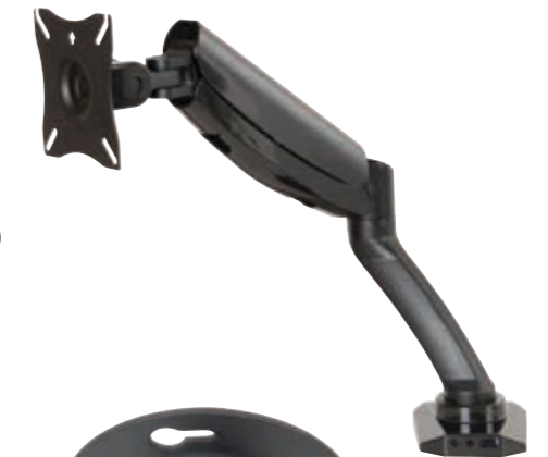
28091T Desktop Monitor Mount Screen Size: 13-27" Max VESA: 100 x 100 Extends: 442mm Tilts: +15/-60° Swivels: +90/-90° Rotates: 360°
