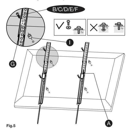
Select the correct size bolts to fit the VESA holes for your TV @/@/@/@/@. Attach the adaptor brackets to the back of the TV by lining up the VESA holes and using bolts ⑤/⑥/⑥/⑥ and the washers ⑥ to fix the TV securely to the adaptor brackets.
